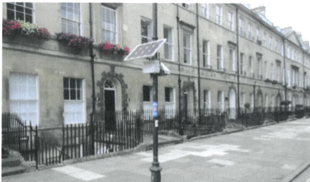
AQMesh Automatic air pollution monitor - Sydney Place, Bath
